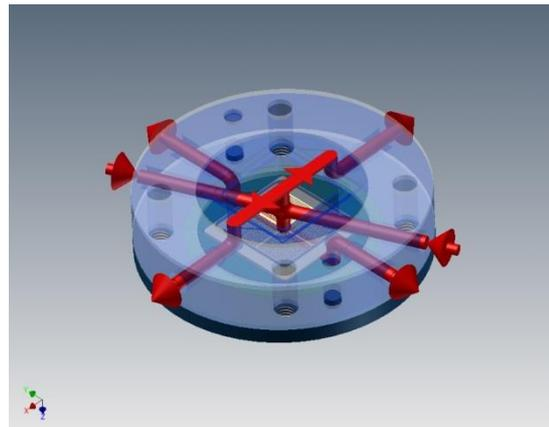
Fig. 4: Flow of medium in perfusion mode. Medium flow is perpendicular to the microcavity array surface.
