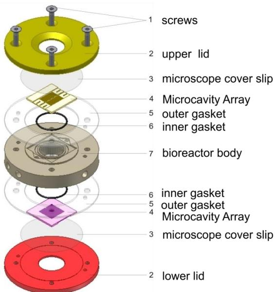
Fig. 3: Microbioreactor for the housing of one or two microcavity arrays.
