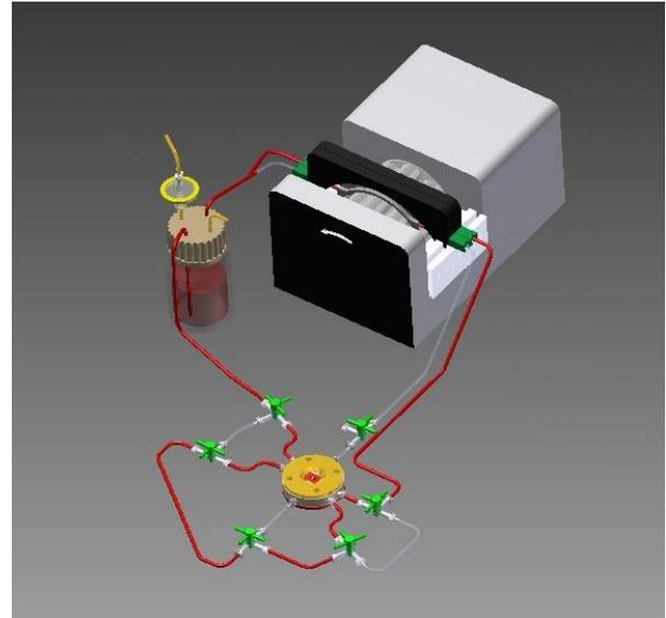
Fig. 6: Bioreactor setup with a closed circulation loop consisting of a medium reservoir, a roller pump and the bioreactor. The medium reservoir can be charged with gas according to standard cell culture conditions or gas mixtures leading to e.g. hypoxia.
