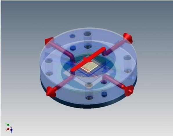
Fig. 5: Flow of medium in superfusion mode. Medium flow is in parallel to the microcavity array surface.
