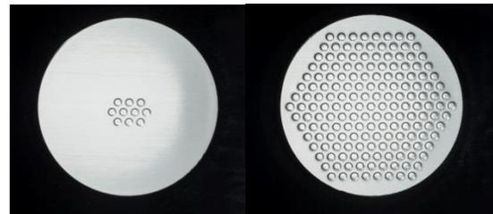
Fig. 2: STATARRAYS<sup>®</sup> Microtiter plate-based microcavity array platform with 169 or 10 microcavities per well, respectively.
