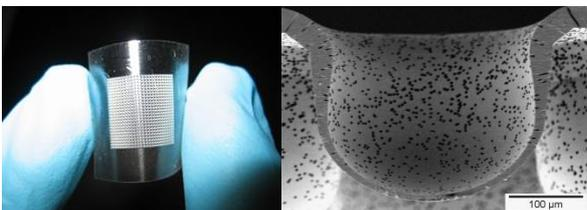
Fig. 1: Left: DYNARRAYS<sup>®</sup> polymer film-based microcavity array. Right: porous microcavity with 3 μm pores. Pore density  $1 - 2 \cdot 10^6$ .
