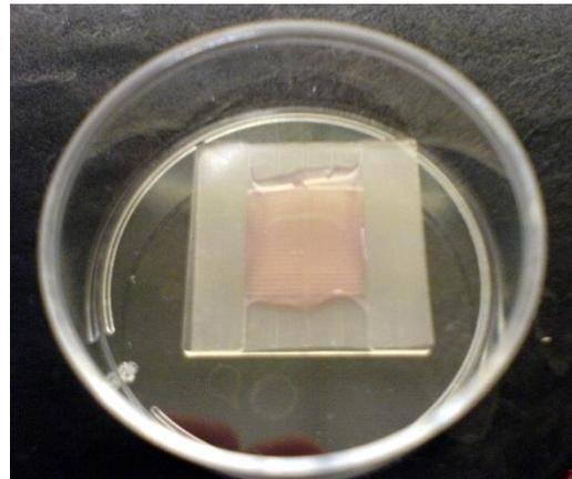
Fig. 7: Droplet formation on top of the DYNARRAY<sup>®</sup> microcavity array.
